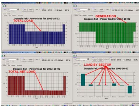
Figure 6: This screen shows the load plan for Iroquois Falls, which is set to run at about 65% of capacity for this 15-minute period in the morning.
