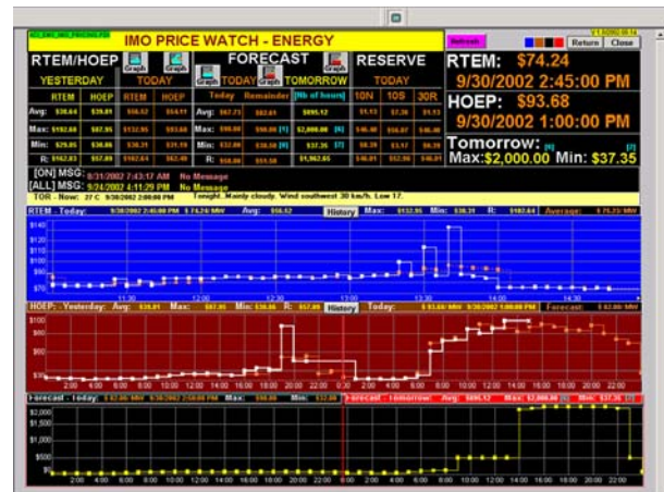
Figure 9: The IMO Energy Price Watch screen brings together all factors that drive MWH pricing in Ontario. This screen includes the Real Time Energy Market (RTM), the Hourly Ontario Energy Price (HOEP), and the pre-dispatch pricing for the next day so that mill operators can better plan the next day's process activities. The message section on each screen lets them highlight information communications among themselves as well.
