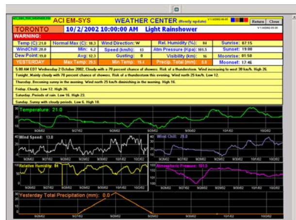
Figure 8: The ACI/EM-SYS Weather Center screen shows all weather factors for the previous day's actual conditions and the current day's forecast, since weather can have a big effect on power consumption.
