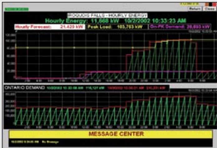
Figure 7: This hourly view of consumption at Iroquois Falls graphs actual vs. planned demand and provides an overview of how the mill is staying with peak limits of the IMO.
