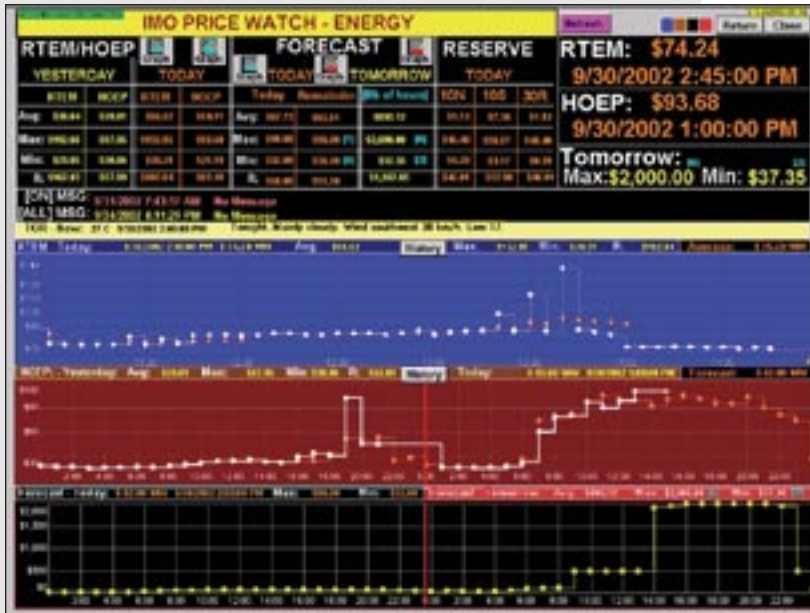
Figure 9: The IMO Energy Price Watch screen brings together all factors that drive MWH pricing in Ontario. This screen includes the Real Time Energy Market (RTEM), the Hourly Ontario Energy Price (HOEP), and the pre-dispatch pricing for the next day so that mill operators can better plan the next day's process activities. The message section on each screen lets them highlight information or communications among themselves as well.
